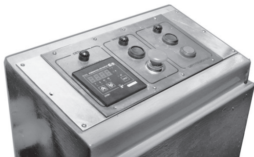
Fig.3. Control panel of the generators
