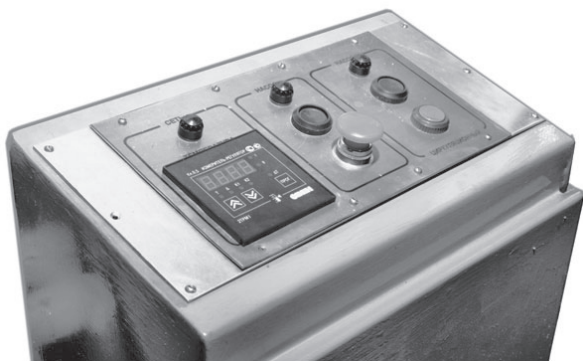
Fig.3. Control panel of the generators
