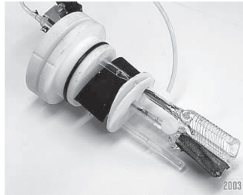
Palladium Reactor. This photo shows a disassembled Cold-Fusion reaction chamber, including the anode and Palladium cathode
