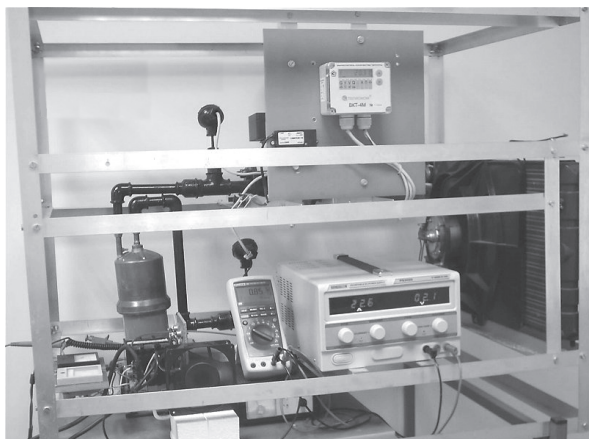
Fig. 4. The experimental device for hydrogen recombination research
