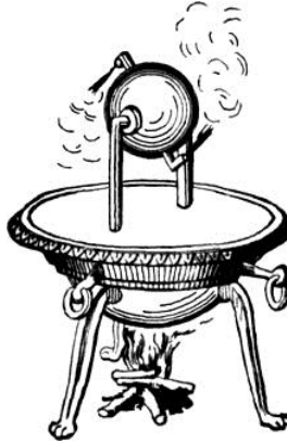
Fig 1. Steam turbine invented by Heron.
