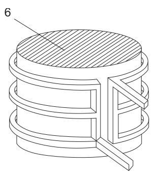
Fig. 2. Three-layered electromagnet with ferrite core
