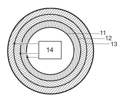
Fig. 5. Three-layered spherical capacitor
