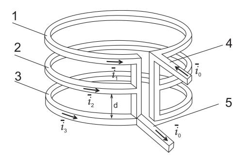
Fig. 1. Three-layered electromagnet
