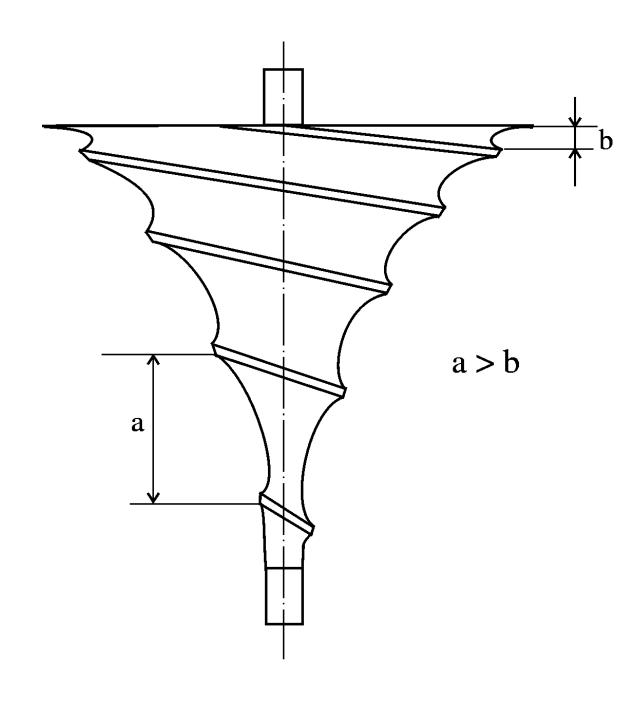
Fig. 3 depicts a variant of the conical case construction with coordinated spirals
